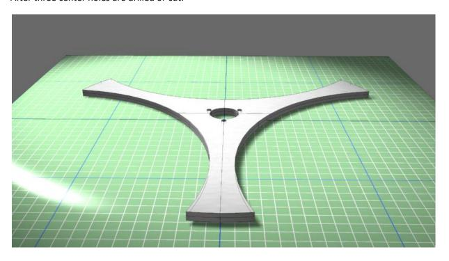
Drill two 0.500" holes on each blade at a distance of 1" and 3" from the tip:
